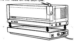
Plug the dc power cord from the BCP-5W into the DC IN 12V Jack at the rear of the receiver.
